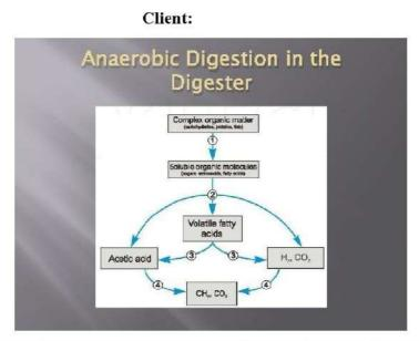
The key process stages of anaerobic digestion
